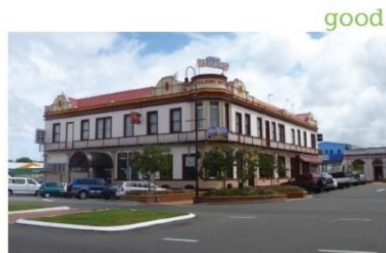
The facade of the Feilding Hotel is a good example as its openings are placed symmetrically, and as a corner building it has doors to both frontages
